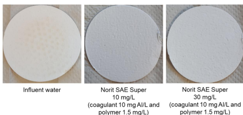
Figure 10. Comparison for the results of filtration tests for the Actiflo® Mini Carb influent, and the effluent with two doses of Norit SAE Super carbon.
