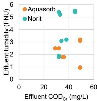
Figure 9. Correlation between effluent turbidity and  $COD_{Cr}$ .
