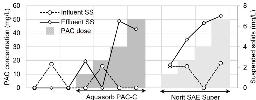
Figure 6. Changes in suspended solids during the PAC trial runs with the pile cloth filter. SS values below detection limit are shown as zero.
