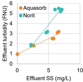
Figure 8. Correlation between effluent turbidity and suspended solids.
