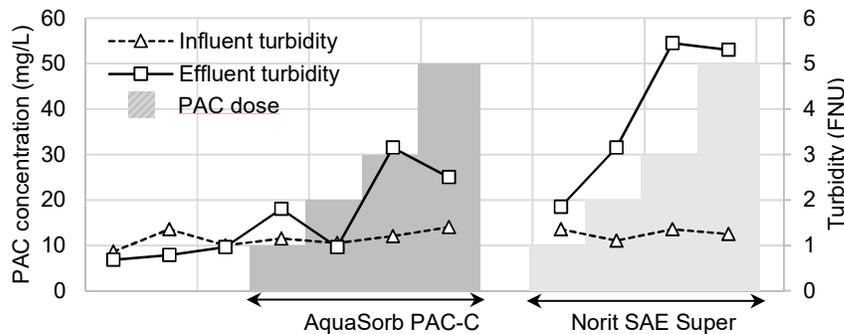
Figure 5. Changes in turbidity during the PAC trial runs with the pile cloth filter.
